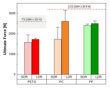
Fig 1. The comparison for ultimate force between 3D printed sockets. The dotted lines indicate the means for TPS and LCS.
