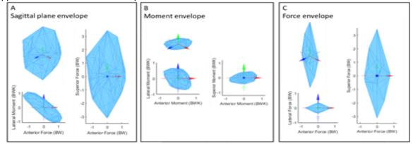
Figure 1. The six-dimensional (6D) failure envelope for the amputated femur with an osseointegrated implant. Box A – three views of the 3D envelope for the sagittal plane. Box B – three views of the 3D moment envelope. Box C – three views of the 3D force envelope. Units: 1 BW = 1 Body Weight = 814 N, 1 BWK = 1 Body Weight applied laterally at the Knee = 125 Nm.
