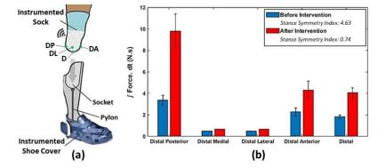
Figure 1. (a) Gait and in-socket sensing system; (b) Example comparison of in-socket forces.
