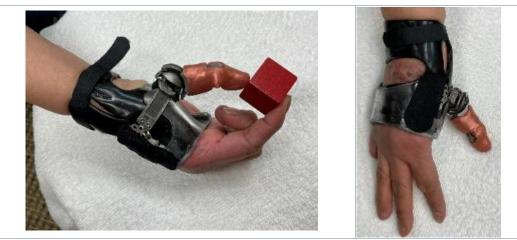
Figure 1: (Left) Prosthesis used in opposition. (Right) Prosthesis used in flat hand posture.
