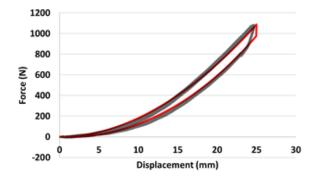
Figure 1: Hysteresis comparison with friction factor. Black: test data, red: model prediction.
