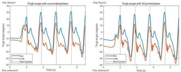
Figure 1. Thigh angle of (L) conventional strap type (R) and 3D printed brace type
