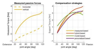
Figure 1. Left graph shows an example of the measured passive forces in the horizontal and vertical workspace measured in a single subject. Right graph shows the different support torque profiles applied in the active elbow support for the same subject. *Note*: Measured-based curve is based on measurement in vertical workspace plus weight component of support interface.
