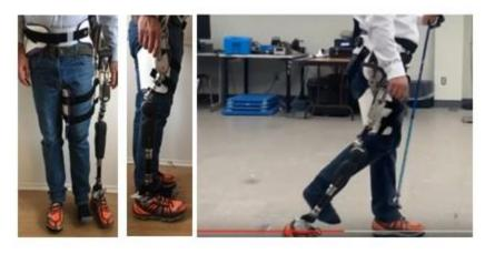
Figure 1: Hip prosthesis simulator using an off-the-shelf hip abduction orthosis and an adjustable adapter.
