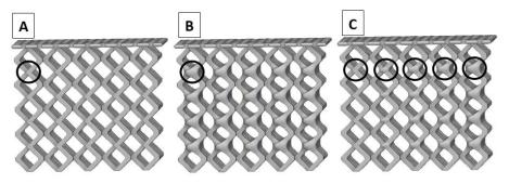
Figure 1. Sample of blend radius settings creating low density (A), high density (B), and transitional density lattice (C).
