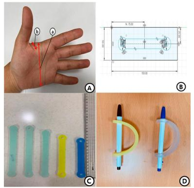
Fig. (A) a. Handbreadth from the MCP joint of the thumb to the MCP joint of the 2nd finger along the surface of the hand. b. Width between the index and little finger. (B) Frame design on the STL file. (C) Five silicon assistive devices according to length. (D) Printing typing and writing integration device.
