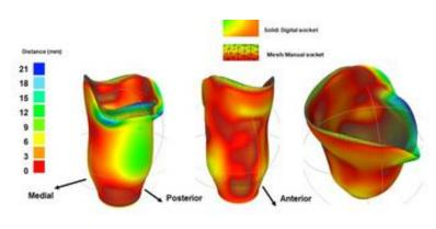
Figure: Manual & digital sockets comparison for participant WPHC01.
