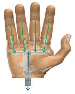
Figure 1. Mechanism of the low-cost hand. Thumb can be rotated to 3 different locking positions.
