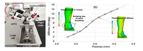
Figure 1: (a) The testing set-up for the measurement of flexural stiffness of AFOs. (b) The effect of thickness on AFO stiffness. The deformed shapes and distributions of mediolateral displacements (in meters) for two selected AFO scenarios are also shown; one scenario where there is buckling (thickness=3.61mm) and one where there is no buckling (thickness=3.60mm).
