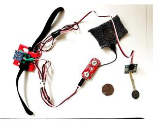
Figure 1 - Arduino, Myoware board, FSR and fabric EMG reference electrode.
