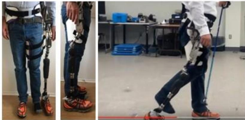
Figure 1: Hip prosthesis simulator using an off-the-shelf hip abduction orthosis and an adjustable adapter.
