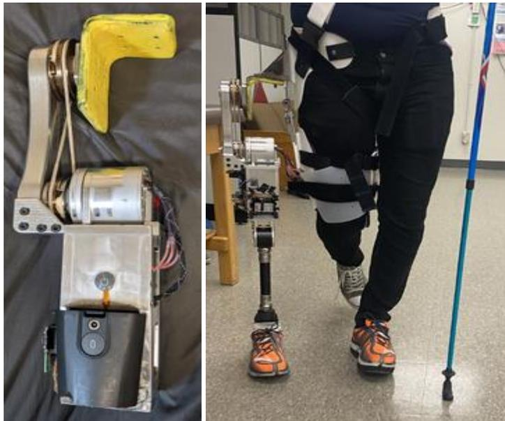
Figure 1. Side mounted power hip joint (left) and joint mounted on prosthesis simulator (right).
